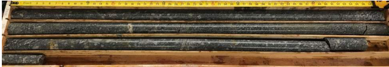
Figure 4-1. Photograph of North Tunnel Engineering Unit 3 Rock Core
