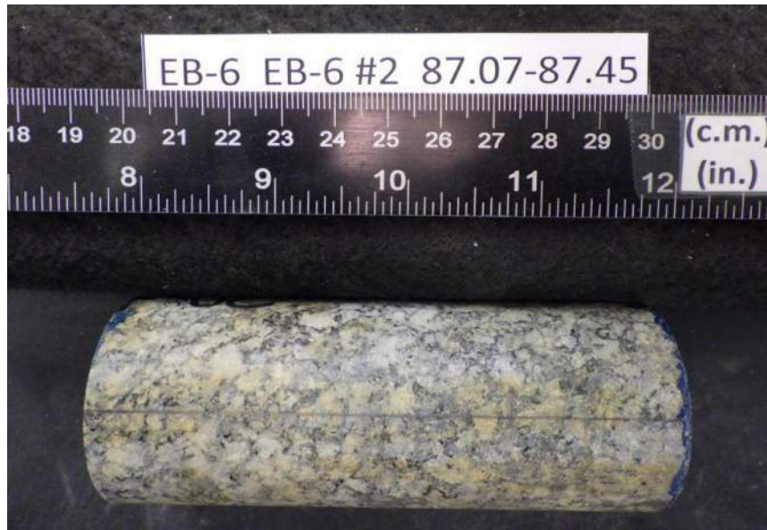
After cutting and grinding
