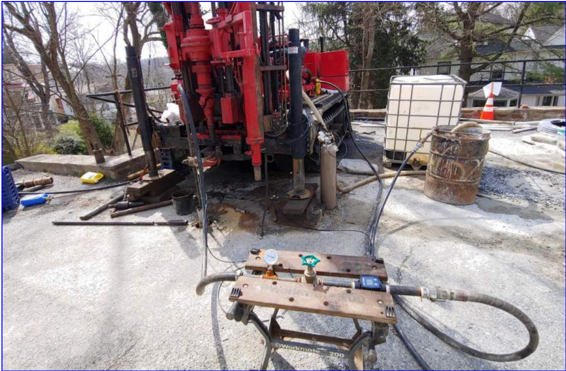
Packer testing setup
